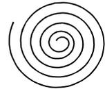
When coil rotates the spring is twisted and it exerts an opposing torque on the coil.
